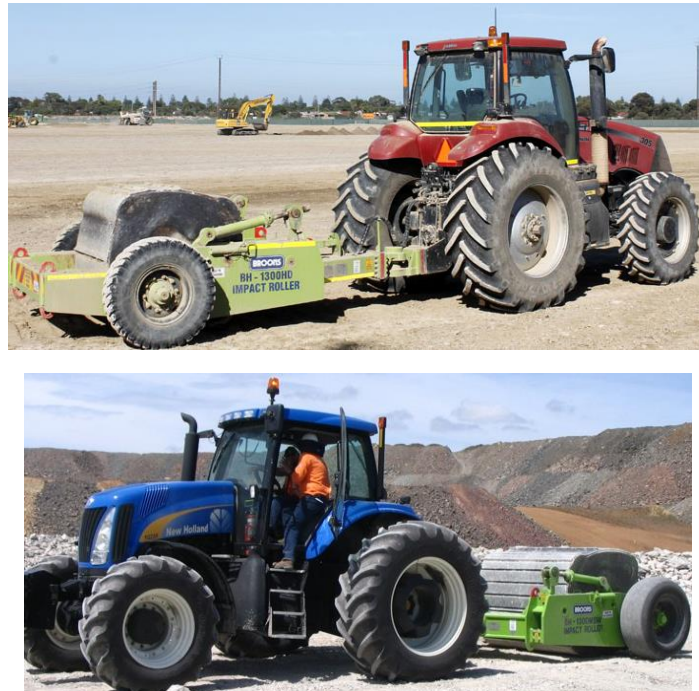
Figure 2: More recent models of Broons 4-sided impact rollers
