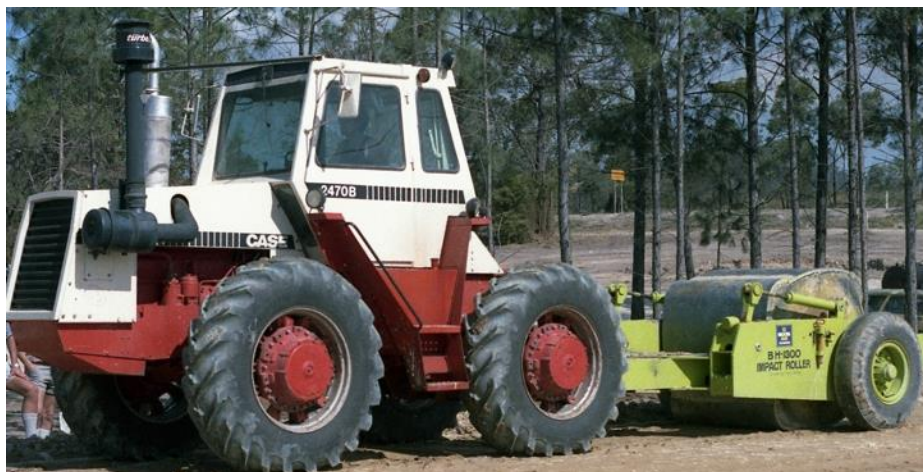
Figure 1: The first Broons impact roller, pictured on site in Australia in 1985
