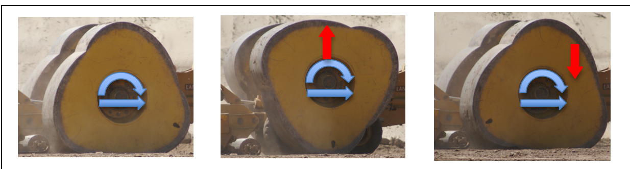
Figure 1. Dynamic Action of Impact Drums
