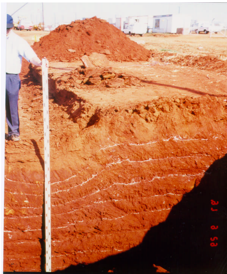
Figure 6: A view of the visual settlement section indicating degree of settlement with depth
